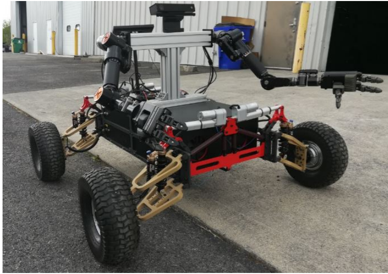
Figure 4.1: The wheeled humanoid robot consists of the TIGER reconfigurable wheeled robot with four EAM and dual arms for high precision manipulation on irregular terrain.
