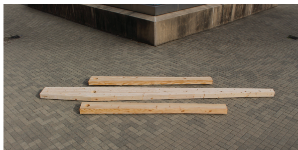
FIG. 21 | All of the bike shelter prototype's wooden members. Each of the project's parts was designed to be fabricated separately before being transported to the site.
