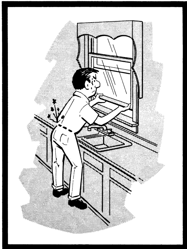
Raising double-hung windows located over sinks or counters places the individual in an awkward position which may result in an accidental slip and fall.
