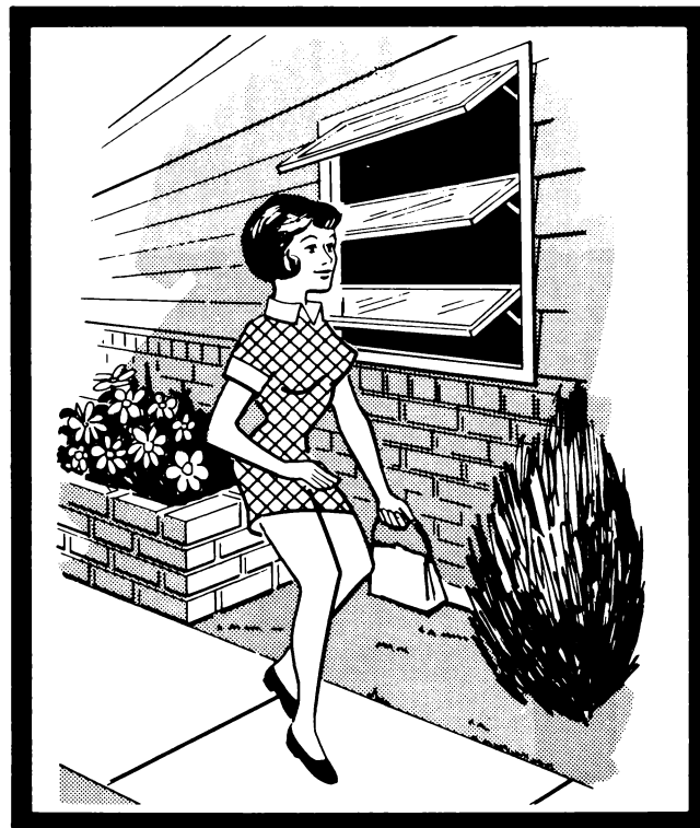
Unprotected projecting windows present a hazardous situation when located so that they open into traffic areas.
