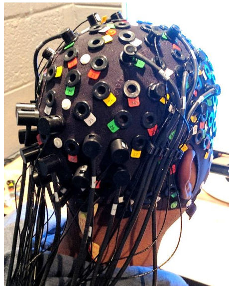
Figure 3. A.) 16x16 channel occipital motor optode layout as displayed in NIRStar software (NIRx Medical Technologies). Red circles denote sources; green circles represent detectors. Purple lines indicate channels. B.) Cap setup in the current study displaying the spring-loaded caps positioned over occipital optodes (image used with participant’s permission).
