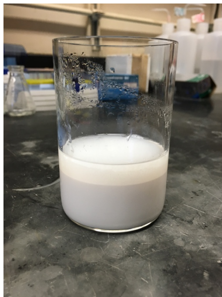
Figure 2.7 Failed poly( l -co-NaSS) polymerization material
