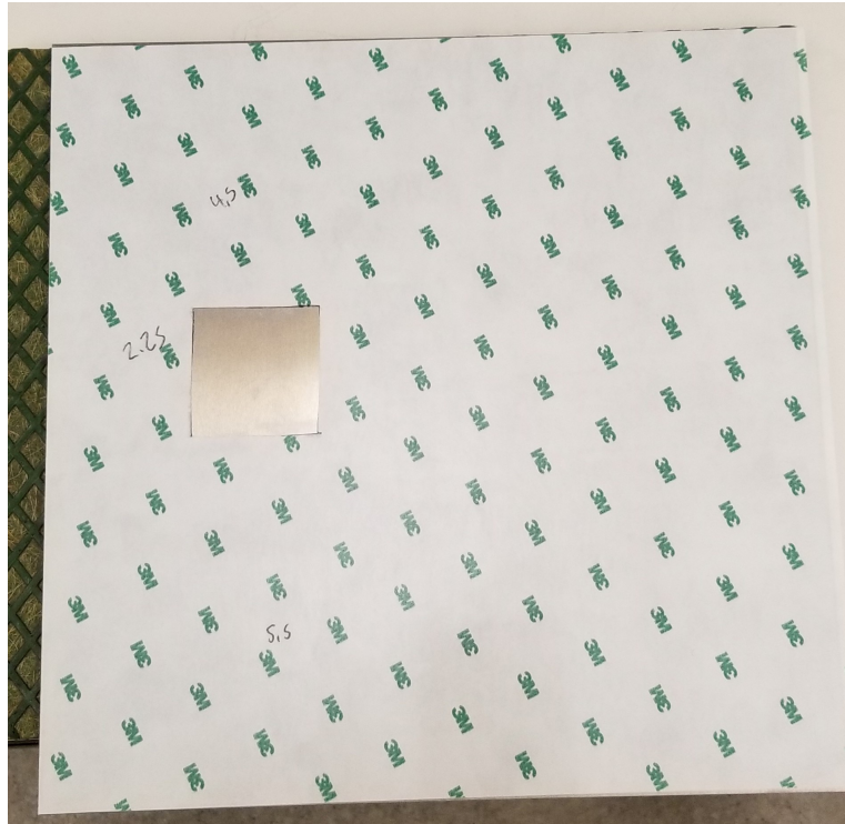
Figure 4.6: The 3M 966 adhesive sheet applied to one side of a metal plate with a 2 in by 2 in square.
