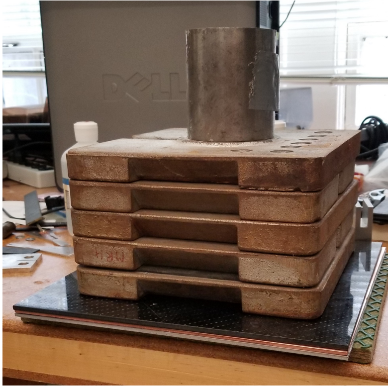
Figure 4.7: Large weights being placed on the two metal sheets in order to evenly bond the two plates together.
