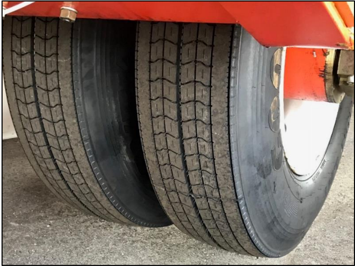
Figure 32 - Wear of HVS Tires
