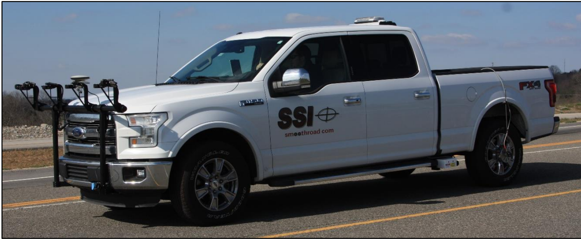
Figure 17 - SSI CS9350 Partial Lane Survey-Profiler
