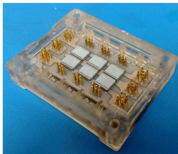
8. Pour silicone gel, degas in vacuum, and cure
