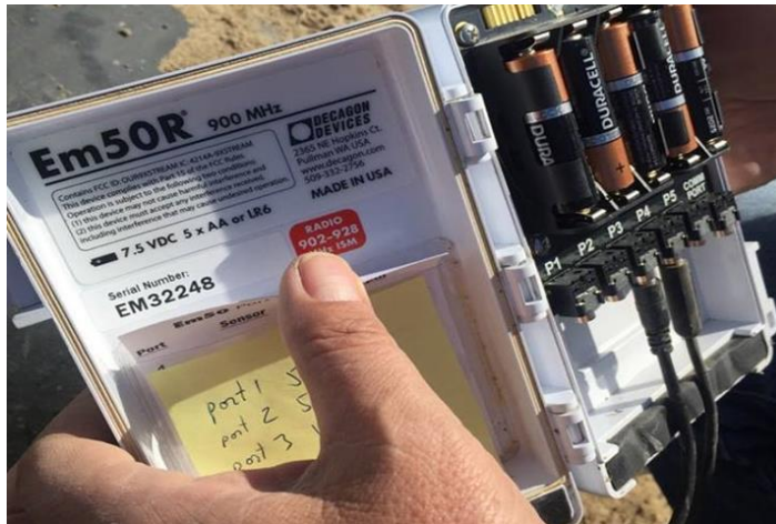
Figure 2: Decagon devices (left) and sensor (5TM) used for the measurement of soil moisture as well as environmental parameter. Eastern Shore, AREC, Painter. 2017-18.
