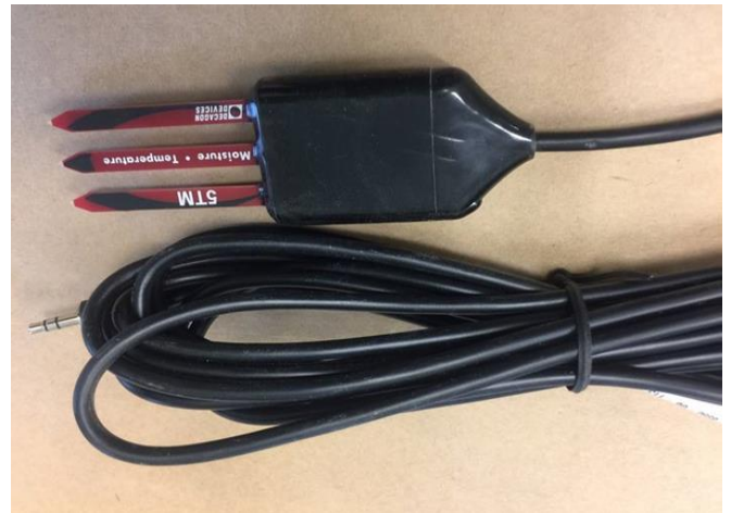
Figure 2: Decagon devices (left) and sensor (5TM) used for the measurement of soil moisture as well as environmental parameter. Eastern Shore, AREC, Painter. 2017-18.
