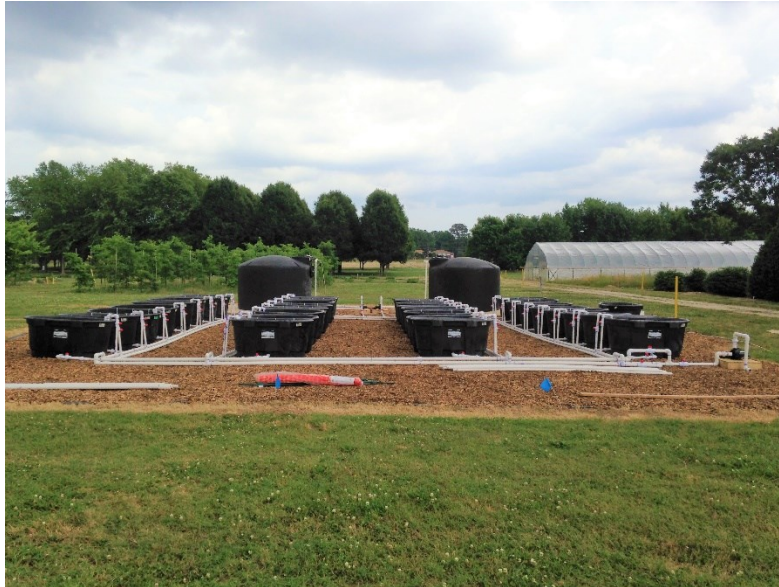
Figure 2.2. Constructed system for FTW mesocosm experiments at the HRAREC.
