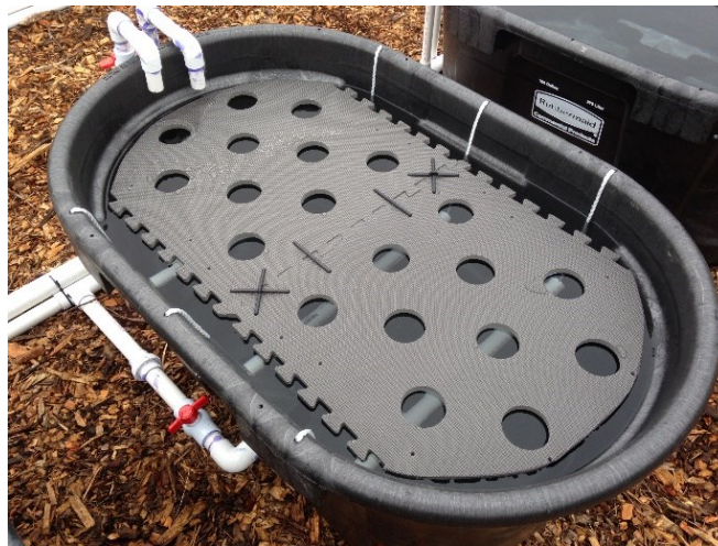
Figure 3.2. Beemat sized to fit mesocosm surface area at operational water levels.
