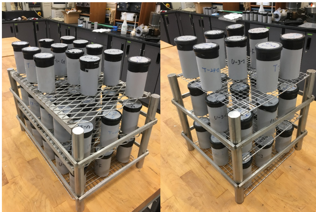
Figure 3-3. Specimen arrangements for curing in the large and small water baths
