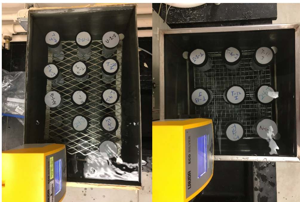
Figure 3-4. Specimens curing in the large and small water baths
