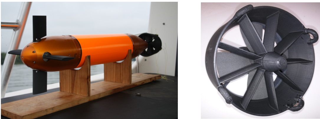
Figure 5.11: Virginia Tech Dragon AUV and base propulsor used in field trials at Claytor Lake in Pulaski County, Virginia
