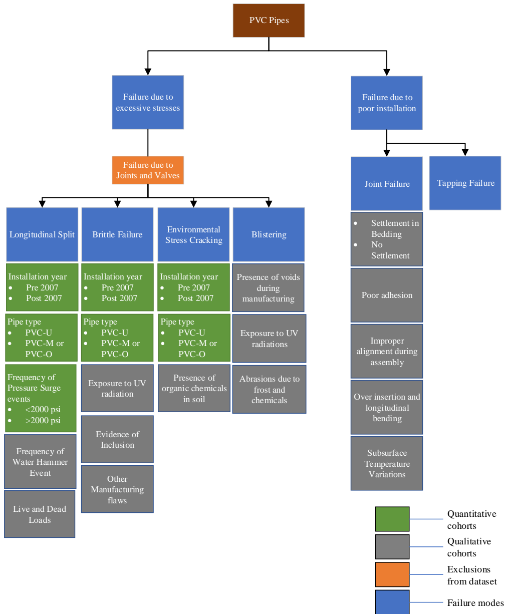
Figure 20: PVC pipe performance analysis framework
