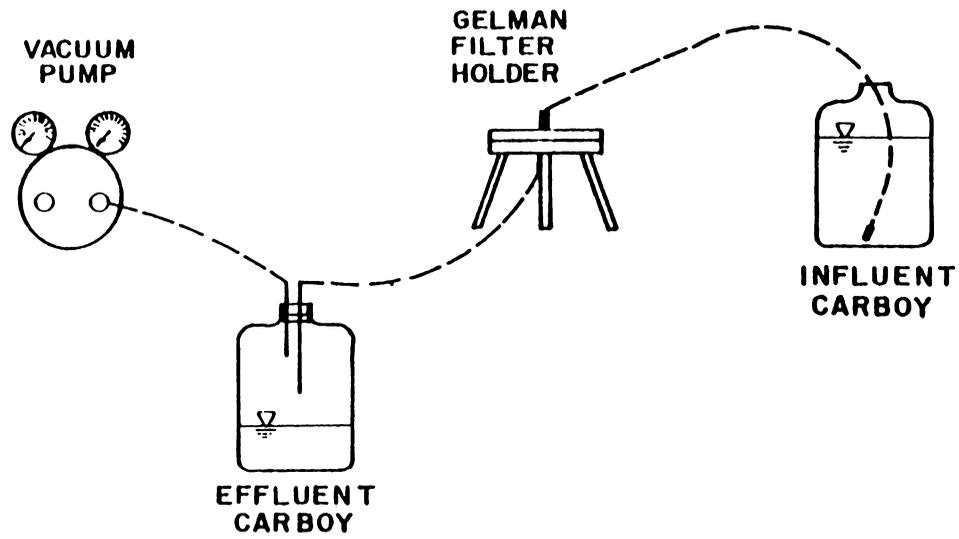
**FIGURE 2. APPARATUS FOR CONCENTRATION WITH VACUUM FILTRATION**
