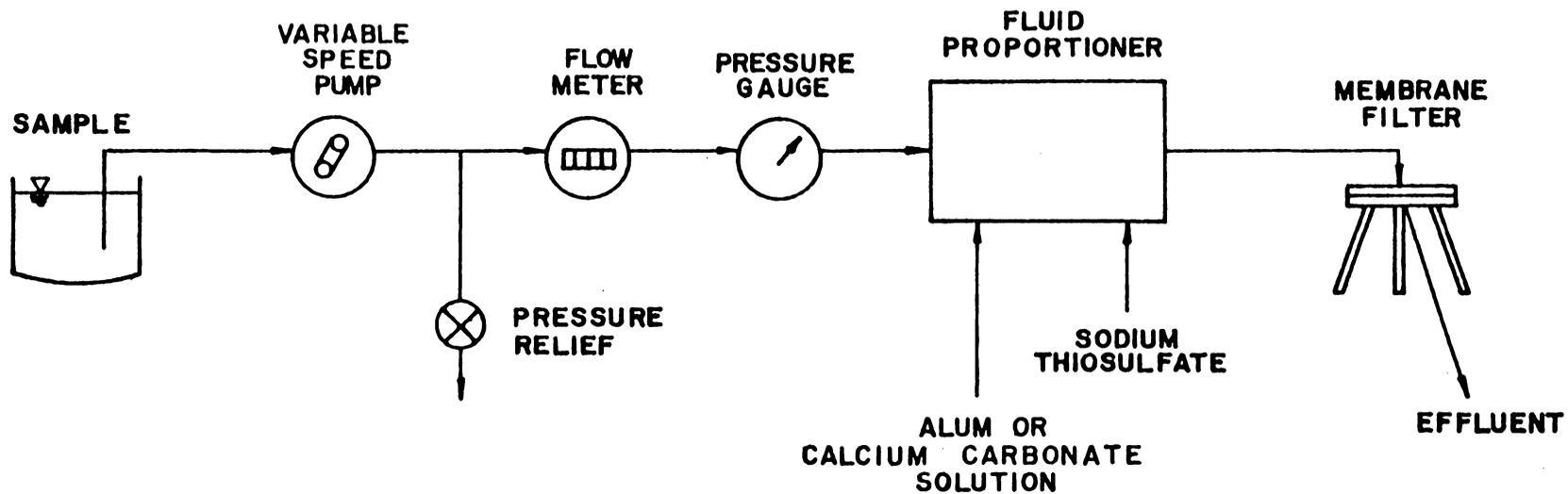
FIGURE 1. SCHEMATIC DIAGRAM OF THE BACTERIAL CONCENTRATOR
