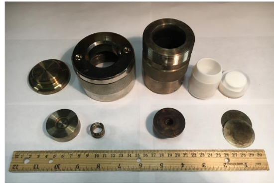
Figure 3.1. (a) Schematic description of hydrothermal synthesis. (b) Picture for autoclave used in hydrothermal synthesis.
