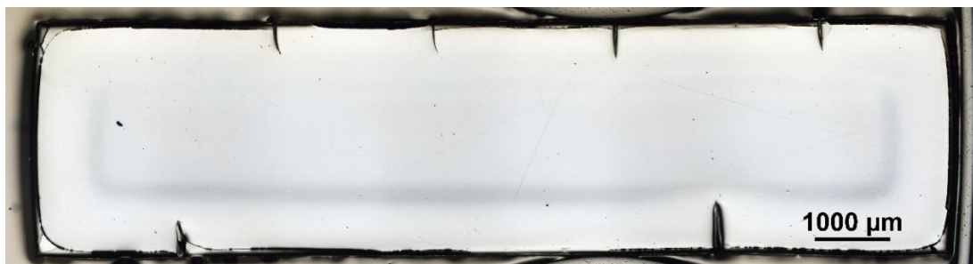
Figure 123: Mounted and polished cross-section after aging for 5000 hours at 250 °C, taken with 2.5x objective lens. The surface layer measured approximately 0.7-0.95 mm thick.
