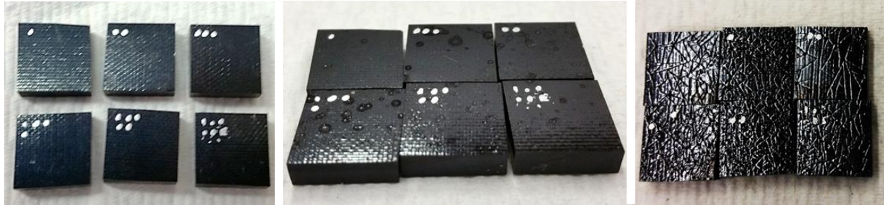
Figure 122: Samples of PN2 cured to 350 °C for 4 hours; aged at 250 °C for 0 hours (left), 720 hours (middle) and 4200 hours (right).
