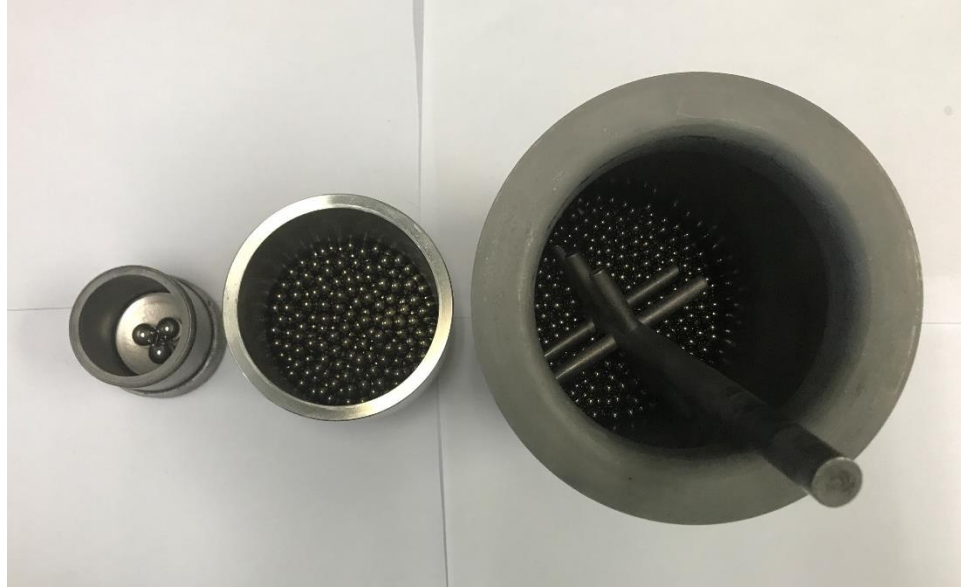
Figure 4. Batch Comparison of Milling Techniques. From left to right: vibratory milling vial, a planetary ball milling vial, and an attritor milling vessel. The containers shown are laboratory scale with larger containers existing for each.
