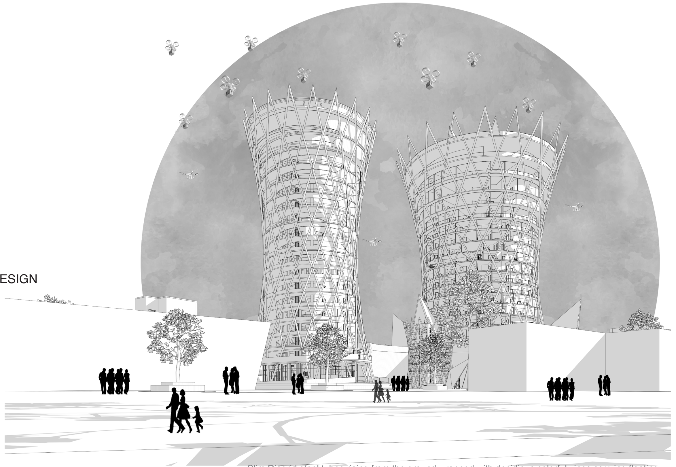
Slim Diagrid steel tubes rising from the ground wrapped with deciduous colorful vines carrying floating floor plates.
