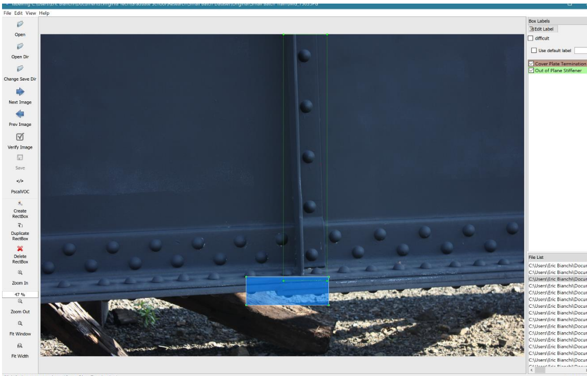
Figure 3.3.1 – Example Window of Labellmg with Cover Plate Termination and Out of Plane Stiffener Annotated.
