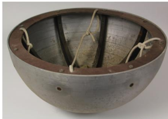
Figure 6. Hemispherical penetrator used during the 1998 and 2000 drop test campaigns (Kellas, 2016)
