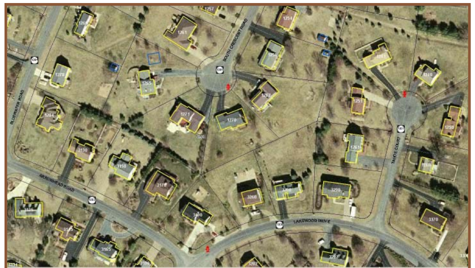
Example of the map display used by 9-1-1 telecommunicators. Included are structures, streets, addresses, fire hydrants, and orthophotography.
