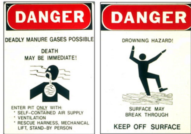
Figure 2. Manure storage safety signage.
