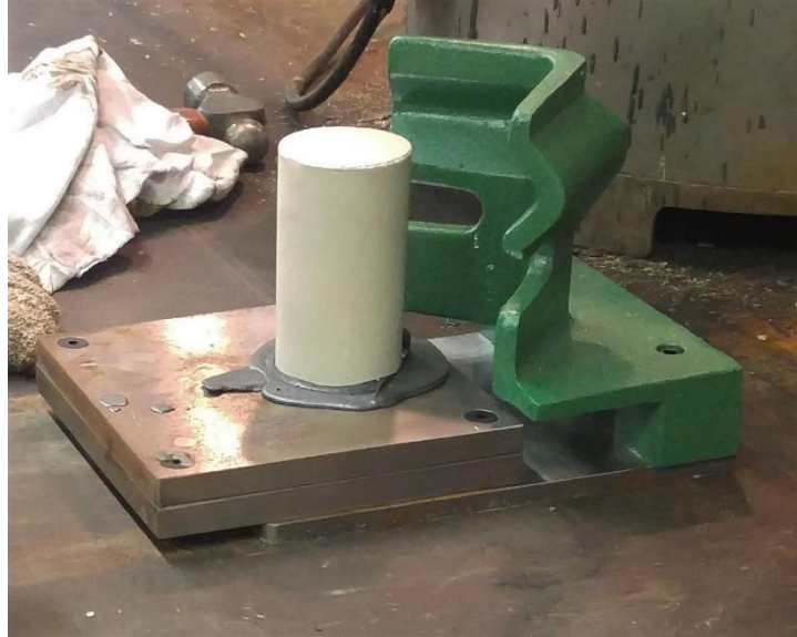
Figure 65: Specimen with dry sulfur cap inside capping plate
