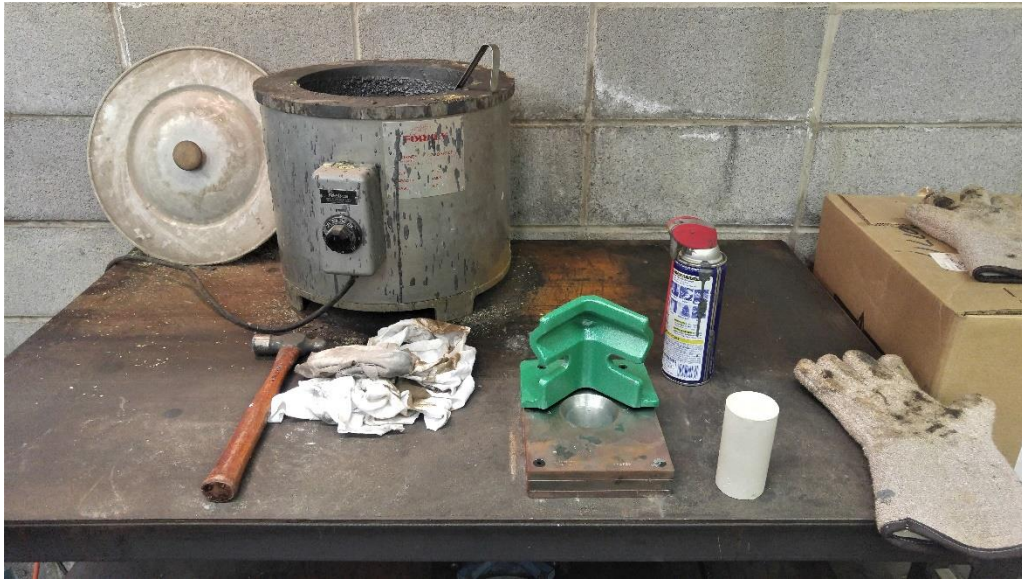
Figure 62: Equipment used for sulfur capping (from left to right): melting pot with cover, hammer with round edge, cloth, Vertical cylinder guide with capping plate for 2" by 4" cylinders, WD-40, cement-treated soil specimen, and heat resistant gloves
