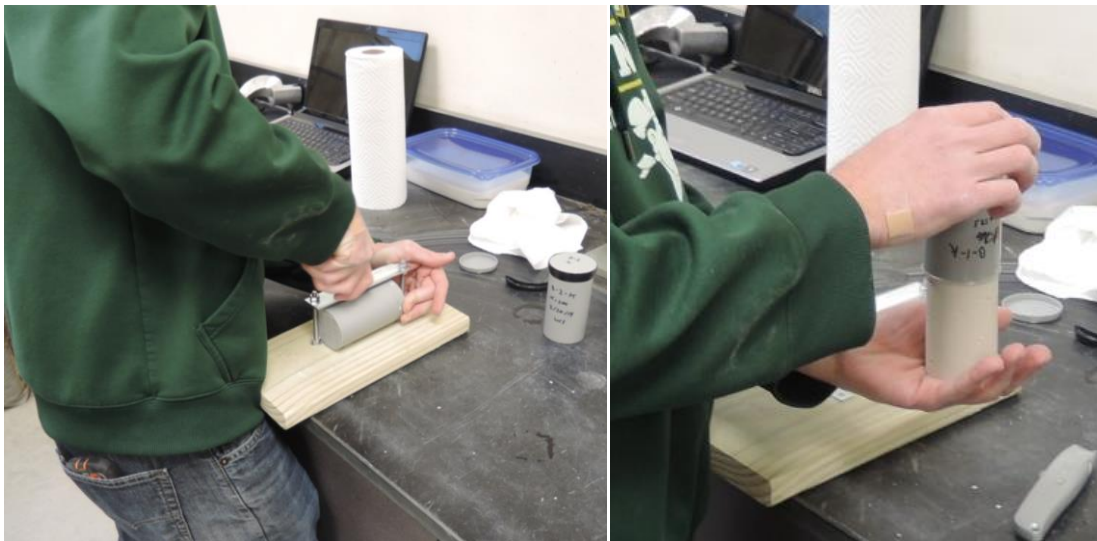
Figure 52: Demolding of a specimen using the jig to make a single cut along the length
