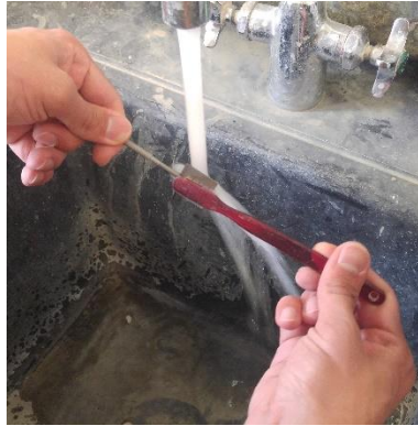
Figure 55: Cleaning of the specimen under running water using a toothbrush
