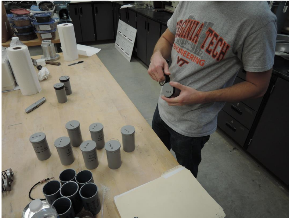
Figure 49: Sealing of the specimens with electrical tape
