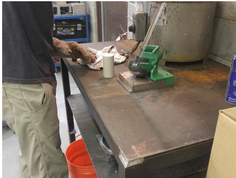
Figure 63: Placing of the molten sulfur into the capping plate with idle
