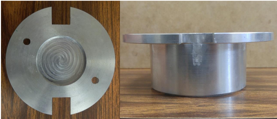
Figure 84: Aluminum base designed for the set up of the device
