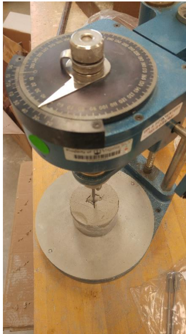
Figure 54: Sheared specimen from a mixture with stiff consistency
