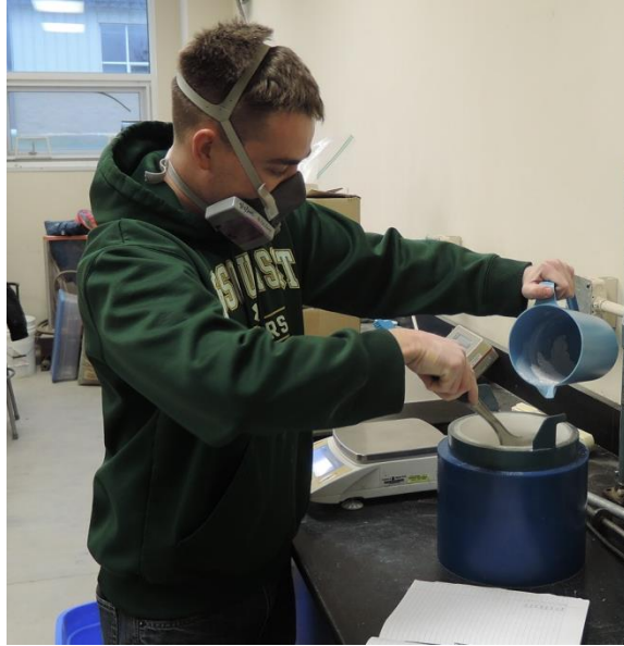
Figure 48: Placing of the dry components into the Jar Mill
