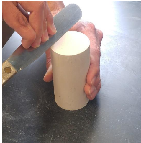
Figure 57: Hand-trimming of the specimen using a straight-edge spatula
