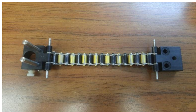
Figure 76: Roller chain and end blocks with 19 rollers (including rollers that are part of the end blocks)
