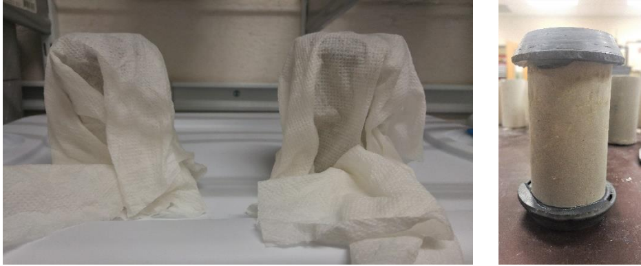
Figure 67: Capped specimens wrapped with moist paper towel (left) and capped specimen before testing (right)
