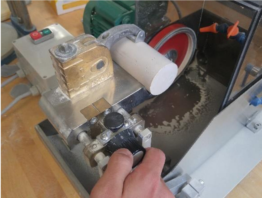
Figure 61: Rotation of the Vernier to move the specimen closer to the grinding wheel
