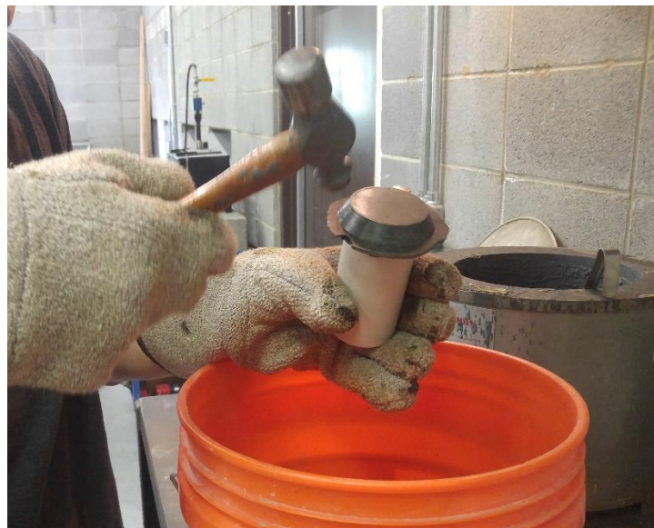
Figure 66: Removal of sulfur residual with a round tip hammer
