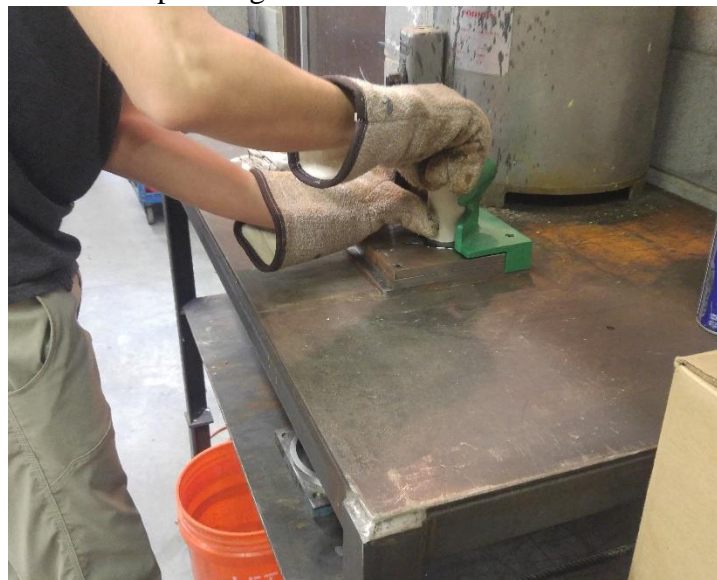
Figure 64: Capping of the cement-treated soil specimen using the capping plate and vertical cylinder guide
