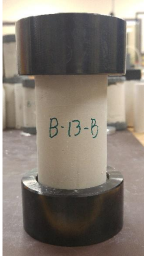
Figure 68: Specimen capped with neoprene pads inside metal caps
