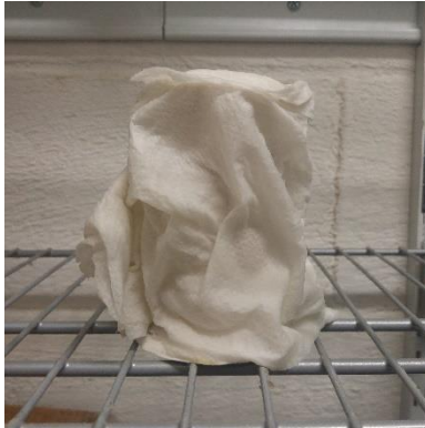
Figure 73: Capped specimen wrapped in moist paper towels
