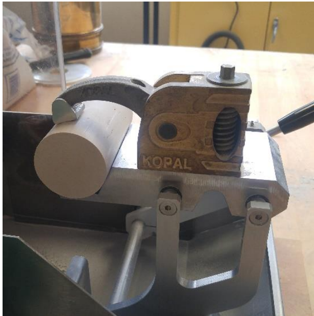
Figure 59: Specimen secured in the v-block with the clamping device
