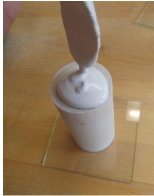
Figure 71: Placing of the mixture on the end-face
