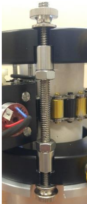
Figure 88: Close view of the alignment posts
