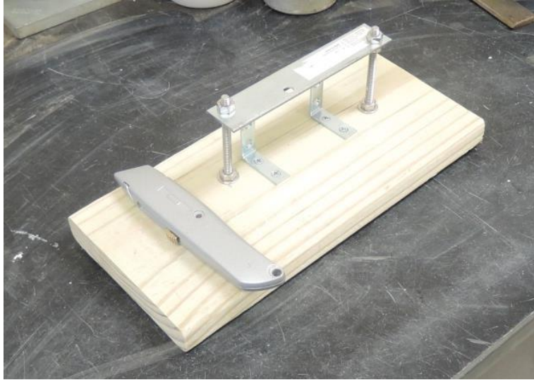
Figure 51: Jig used to demold the specimens and utility knife
