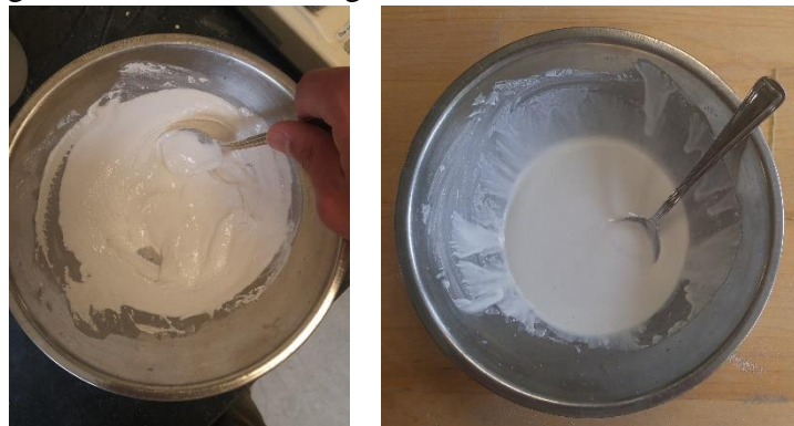
Figure 70: Mixing of the gypsum-water mixture with a spoon
