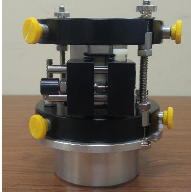
Figure 86: Top collar secured on the specimen with the dowels
