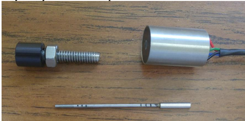
Figure 78: Displacement sensor components (left to right) positioning stem, sensor rod, and sensor body
