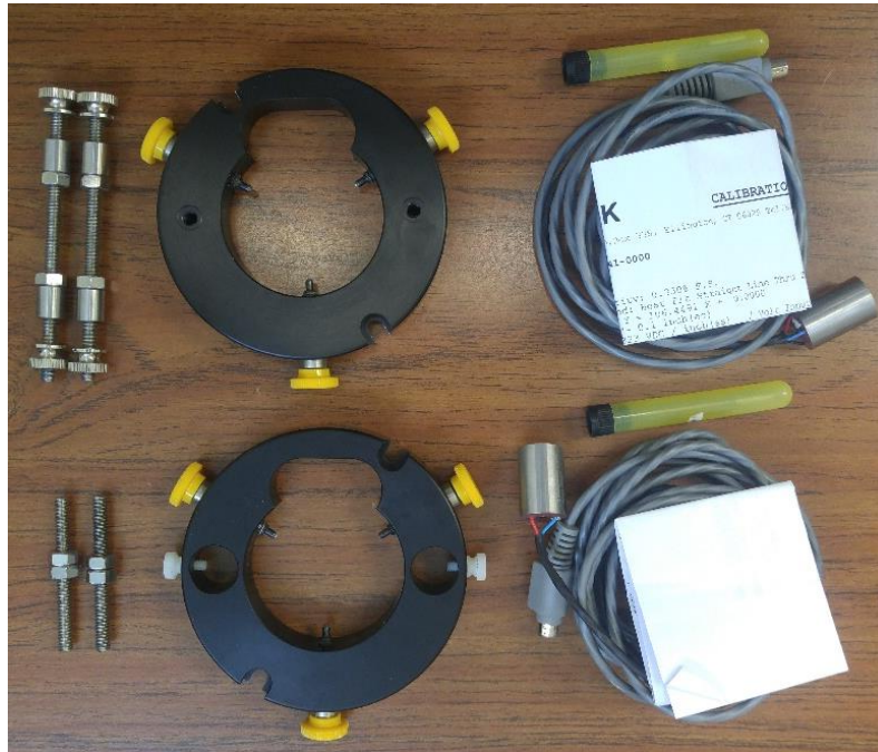
Figure 82: Components of axial strain measurement device (from left to right) collar alignment posts (top left), displacement sensor rod stems (bottom left), lower and upper collars with spring loaded dowels installed, displacement sensors.
