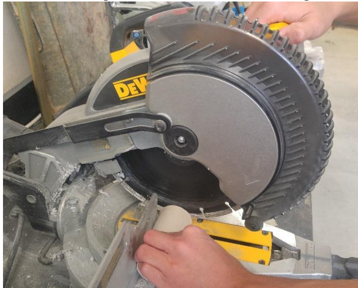
Figure 56: Sawing of the end-face
