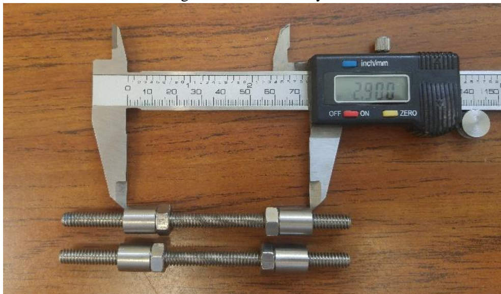
Figure 83: Collar alignment post adjusted for a gage length of 2.9 inches
