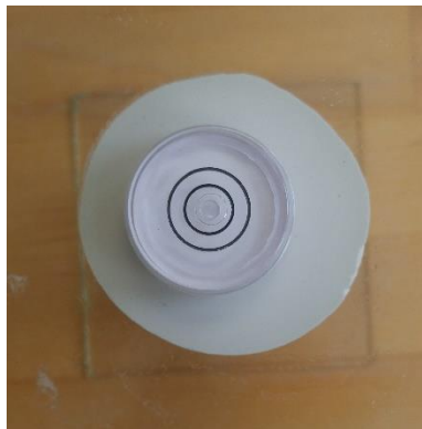
Figure 72: Capping of the specimen with bullseye level
