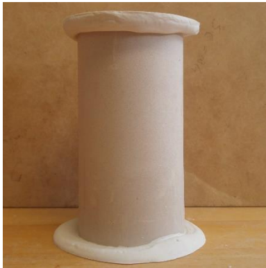
Figure 74: Capped specimen prior to test
