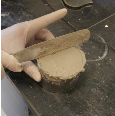
Figure 53: Screeding of the mix to make the specimen for testing
