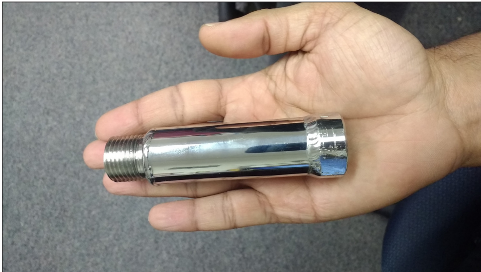
Figure 3: An NLP water “conditioner” that claimed to soften water without any treatment chemicals did not perform as advertised in a battery of laboratory tests conducted by our team.
