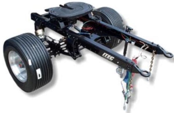
Figure 5-5. An example of a C-dolly. ( http://itec-inc.com/dolly/c-dolly.html , accessed August 2017)
