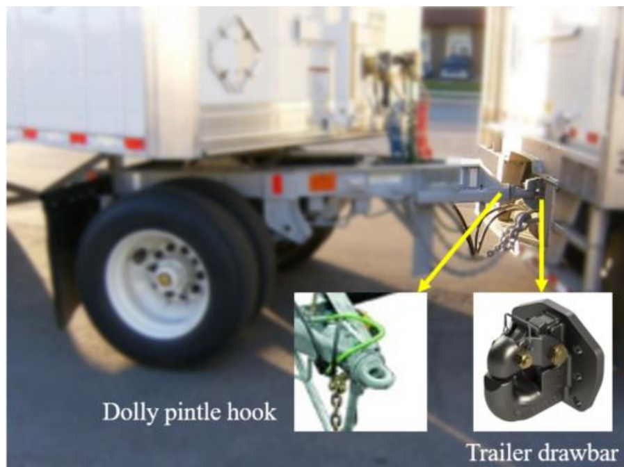
Figure 5-3. An example of pintle couplings commonly applied to trucks in an A-train configuration.
