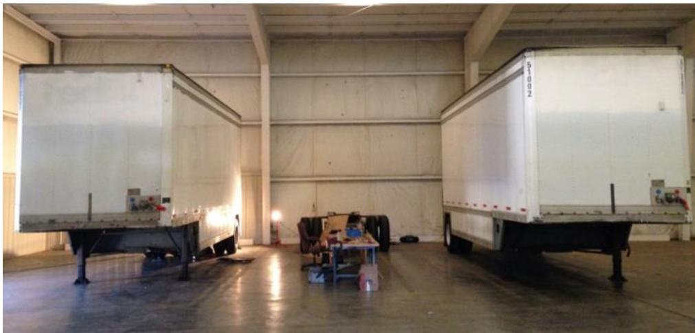
Figure 7-2. Two identical 28-ft drop-frame semitrailers used for testing.
