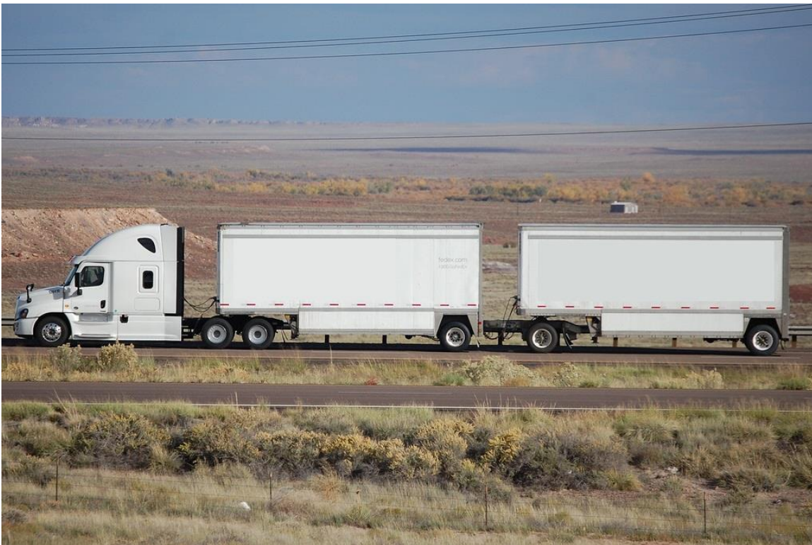
Figure 6-1. A typical 28-ft A-train double that is commonly operated in the United States. ( https://www.flickr.com/photos/scottash/15096687894 , accessed August 2017)
