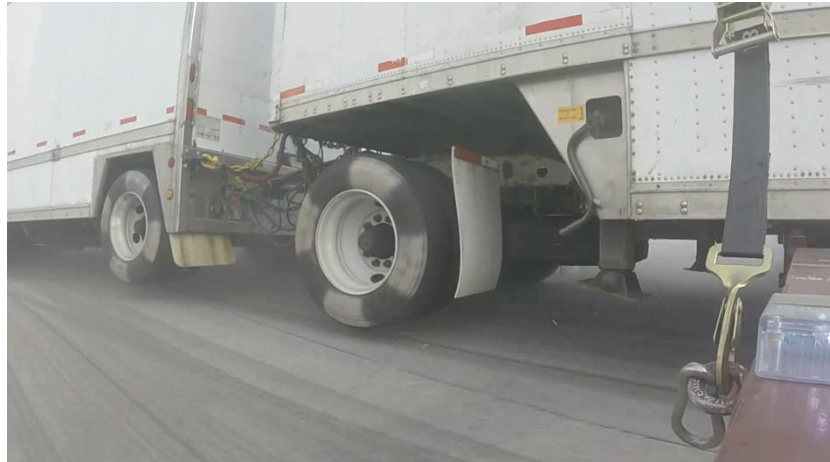
Figure 7-20. Wheels were lifted when outriggers contacted the ground.
