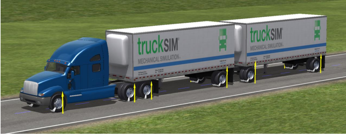
Figure 6-6. The complete 28-ft A-train double model developed in TruckSim.
