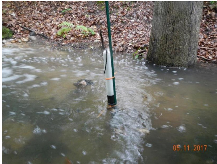
Figure 4.5: Rhodamine WT dye sensor in the bottom pool of the Broad Creek SPSC during the May 11, 2017 controlled flow releases. Photo by Tess Thompson (2017), used with permission.
