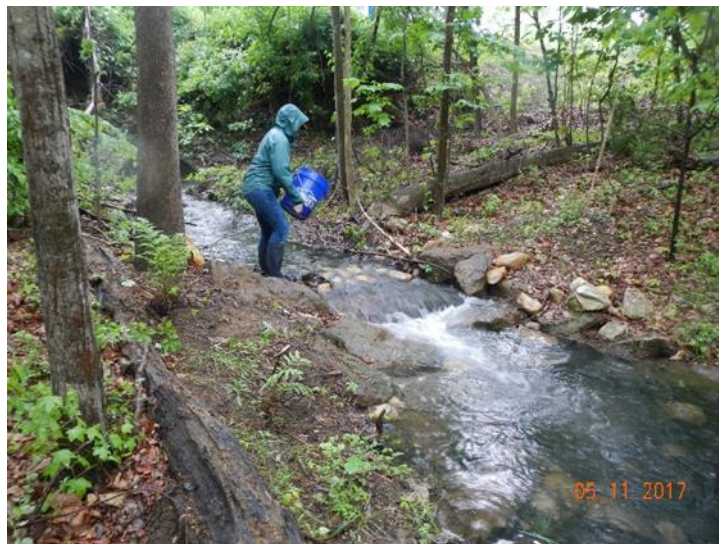
Figure 4.9: Flow over rock weirs at the Broad Creek SPSC on May 11, 2017, just prior to dye release.
