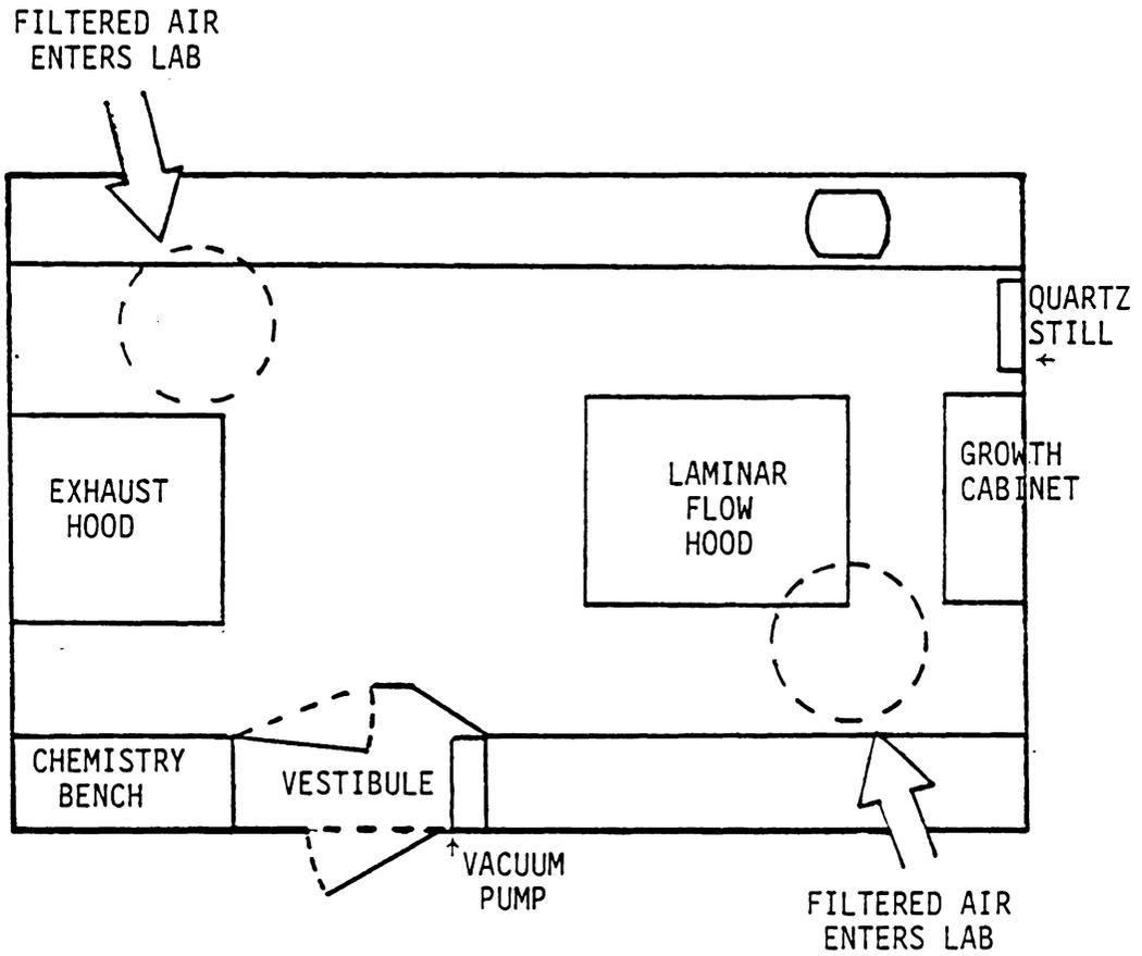
Figure 1. Schematic diagram of class 10,000 clean laboratory.
