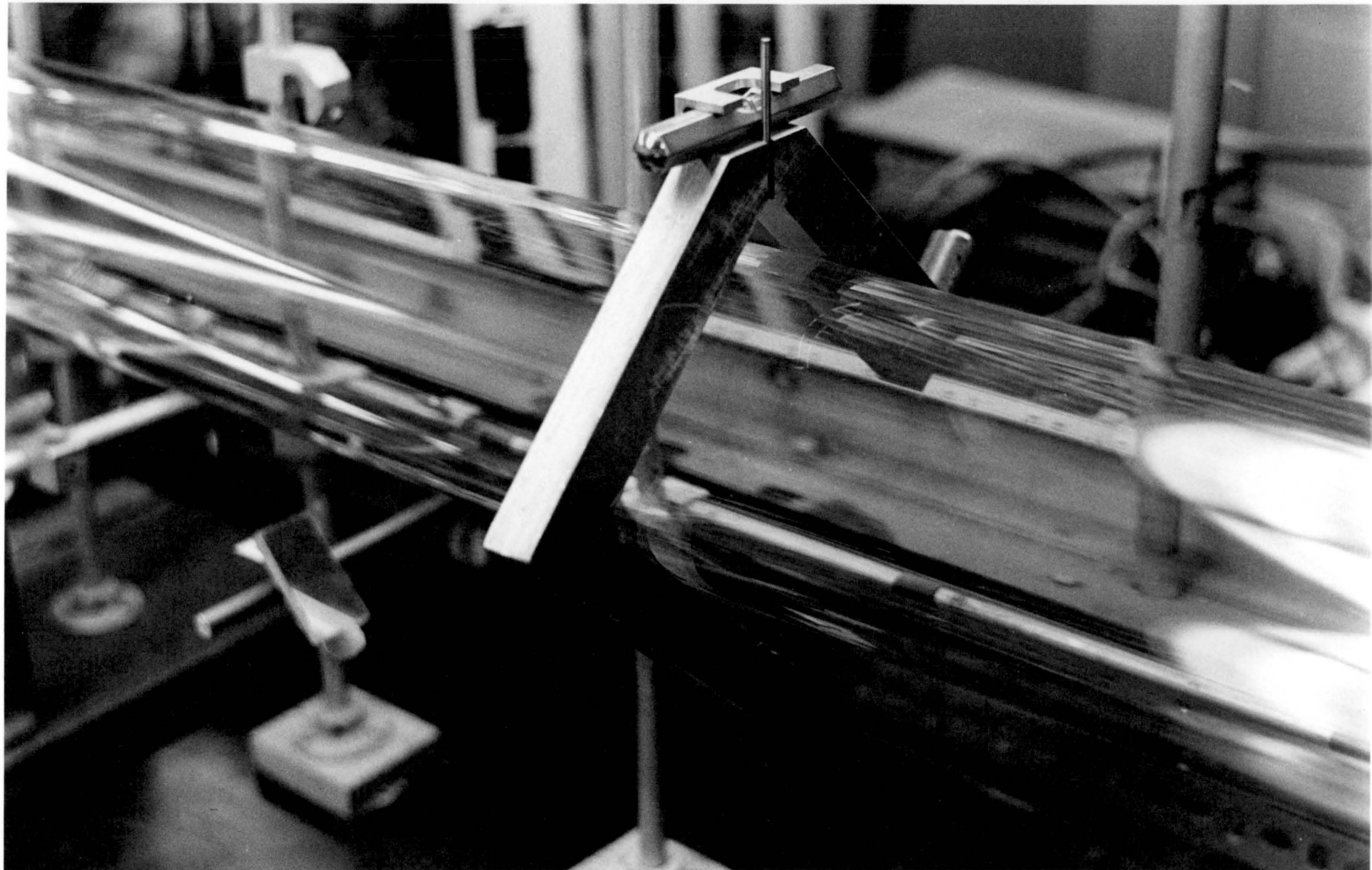
Figure 32. Tool for Locating the Shock Tube Centerline for Adjustment of the Schlieren Mirrors.
