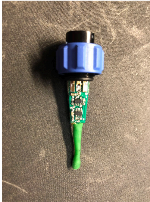
Figure 2.6: Analog Ultrasonic Microphone(monomic, Dodotronic, Rome, Italy)
