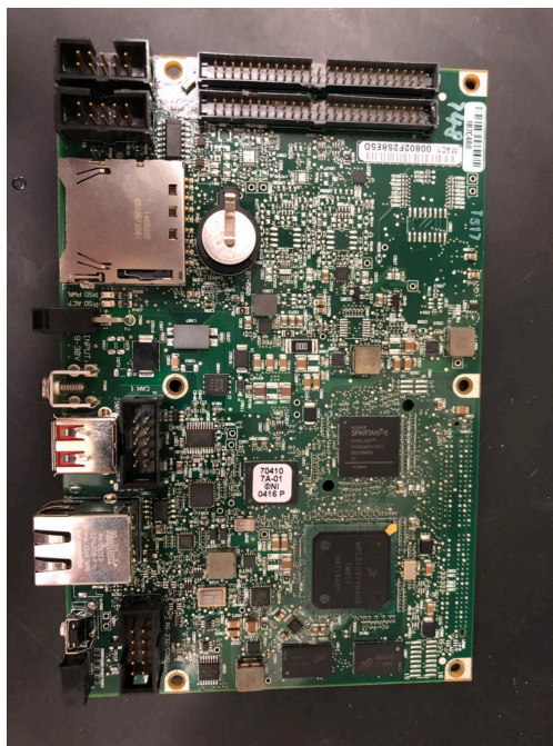
Figure 2.7: National Instrument Pixel 6351 Multifunction Input and Output Device (PXI 6351, National Instruments, Dallas, Texas, USA)
