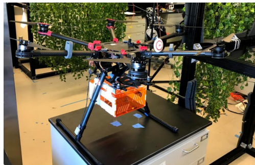
Figure 2.9: Sonar Head on a DJI S900 Drone (S900, DJI, Shenzhen, Guangdong, China)
