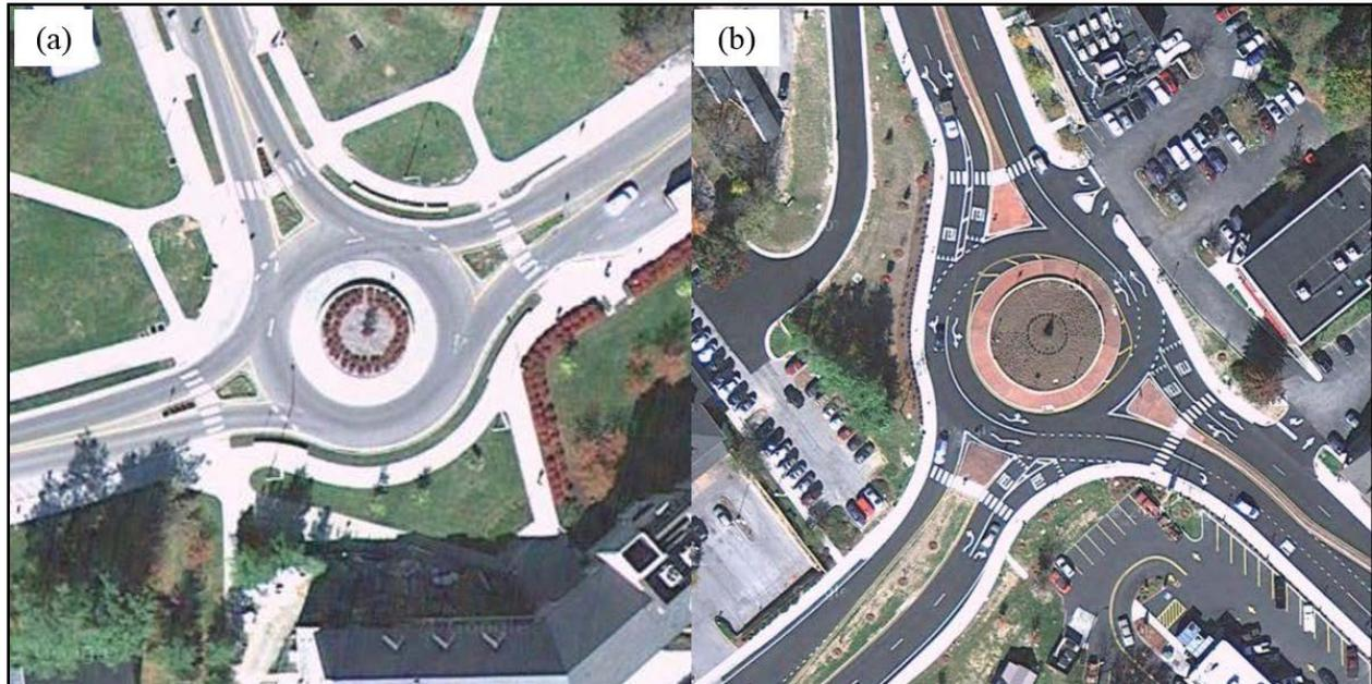
**Figure 1. Photo. (a) Single-lane roundabout and (b) two-lane roundabout used in study (Google Maps, 2016).**
