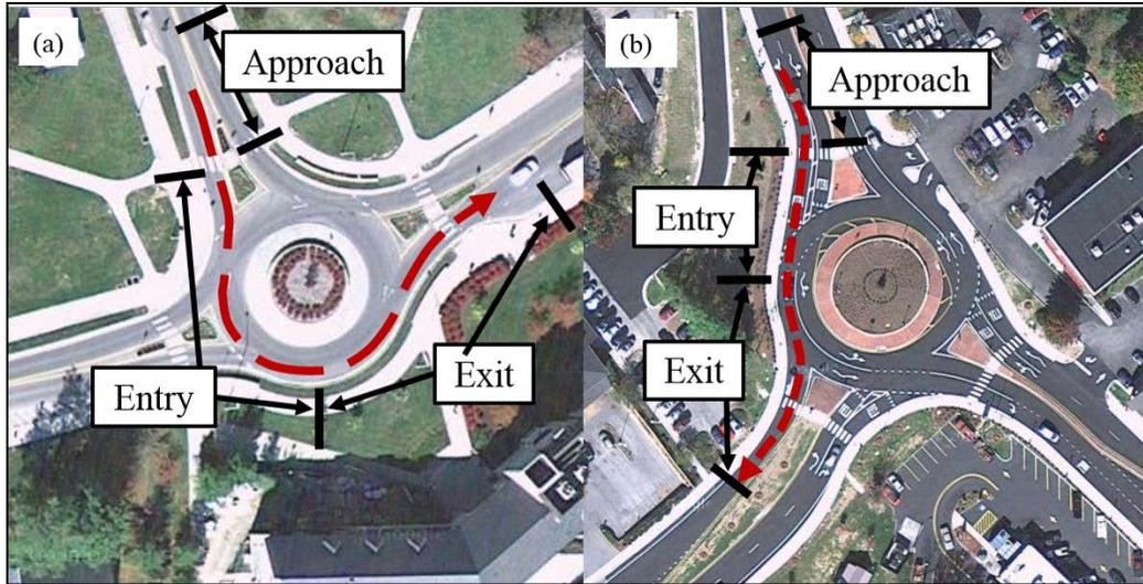
**Figure 2. Photo. Vehicle location for both roundabouts: (a) left turn; (b) right turn (Google Maps, 2016).**
