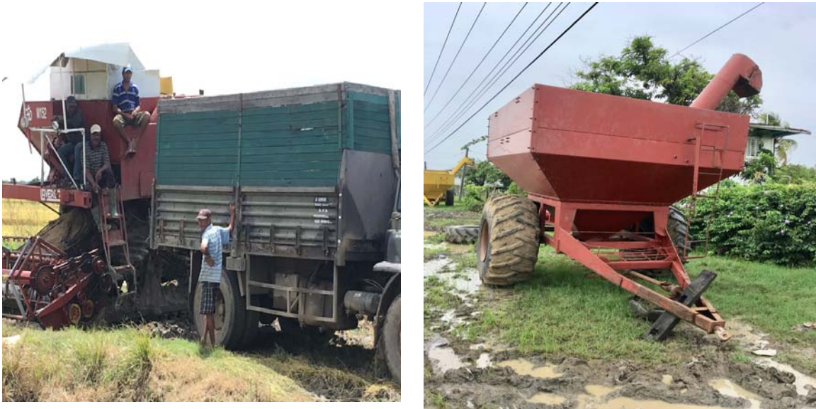
Figure 6.3 Combine harvester and transport truck (left) and grain cart (right) Photo credit: Author
