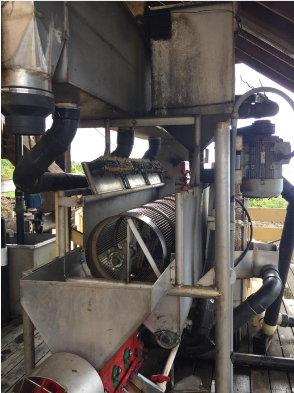
Figure 2: Fermentation tank used to ferment coffee parchments after removing the fruit skin is soaked in water for 14 to 24 hours
