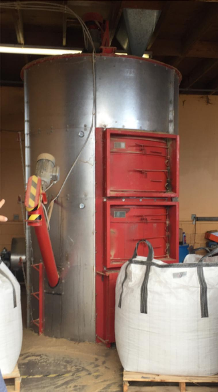
Figure 5: Demucilager used to remove cherry skin and mucilage prior (Semi- wet) of drying the coffee parchments
