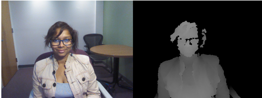
Figure 1.3: Example RGB image (left) and corresponding range image (right) captured by the Kinect. This example shows the artifacts in depth maps resulting from glasses in structured light methods.
