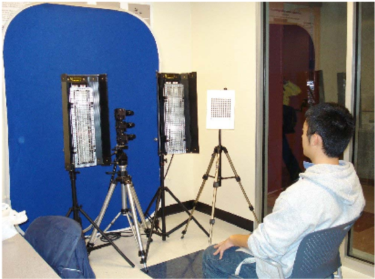
Figure 2.3: 3D dynamic imaging system setup for BU-4DFE [5].
