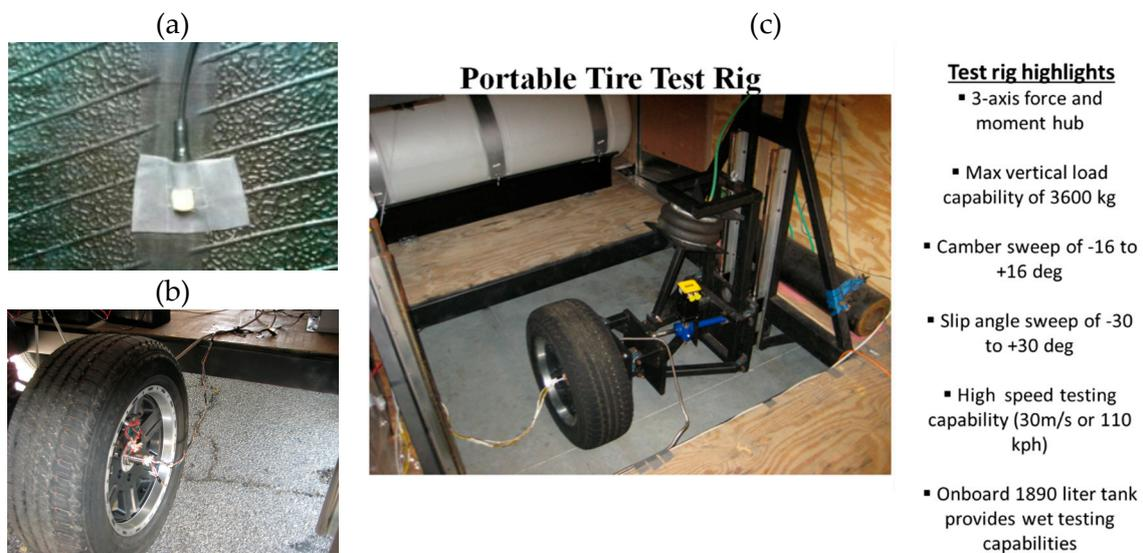
**Figure 3.** Smart tire application: (a) Sensor mounted on the tire footprint centerline; (b) instrumented tire assembly with a high-speed slip ring; (c) mobile tire test rig.
