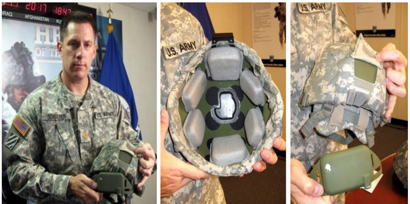
Figure 28. PEO Soldier's Major William Schaffer displays a Kevlar helmet with externally mounted sensor to collect blast data, at left; the sensor, in center; and at right, the internally mounted helmet sensor. Army News, Fort Belvoir, VA, 7 January 2008. (See Fair Use Determination)
