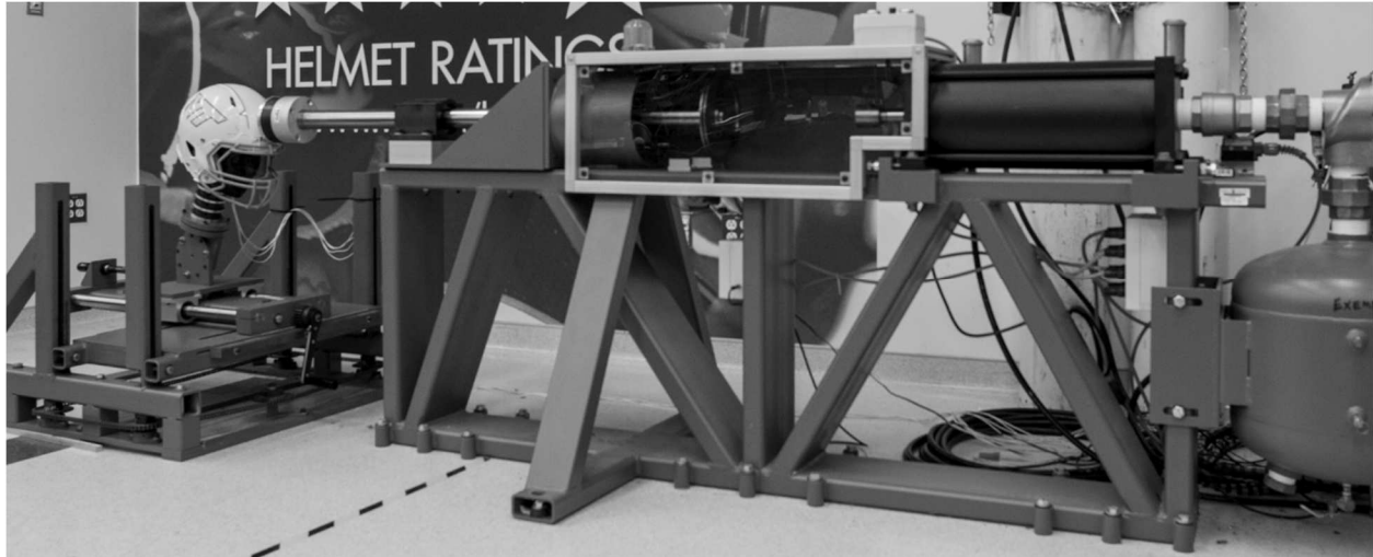
Figure 6.2: Pneumatic ram linear impactor. A helmeted headform and neck assembly are mounted on the linear slide table. This system has the capacity to test speeds up to 11 m/s.
