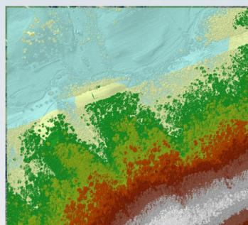
3. Convert TIN dataset to TIN triangles, and select triangles that have slope degrees greater than or equal to 70
