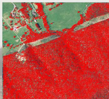
4. Dissolve Step 3's output, and select triangles that have shape areas greater than or equal to 50 ft<sup>2</sup>
