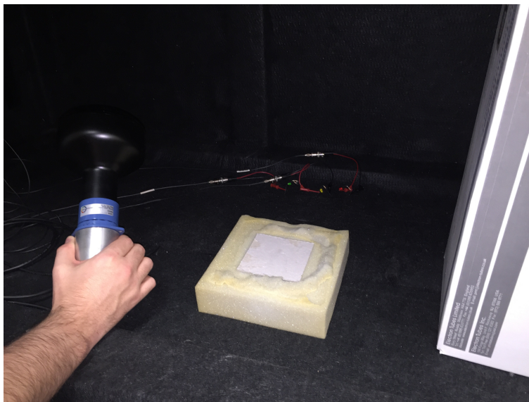
Figure 5.15: The dark box with LEDs and PMT used in the nonlinearity measurement.
