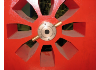
(b) Photograph of the tungsten beam collimator after installation into the first collimator.
