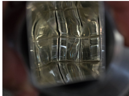
(b) Downstream luminosity monitor light guide after Q_{\text{weak}} run. Quartz at the bottom and light guide both look clear.
