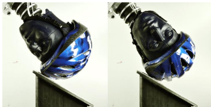
Figure 3.2. Headform orientation for a frontal impact (left) and a temporal impact (right). The anvil was sloped 30° from the horizontal to generate appropriate normal and tangential incident
