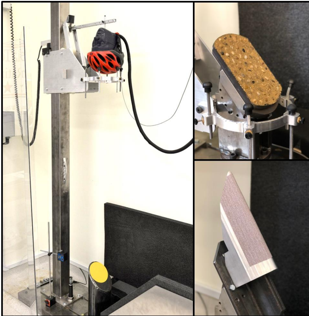
Figure 10.2. Oblique impact drop tower containing angled anvils used for reconstruction testing. A variety of impact surfaces were employed as needed to simulate different accident conditions. A sandpaper-coated steel anvil simulates a smooth road condition (left), while a rough anvil
