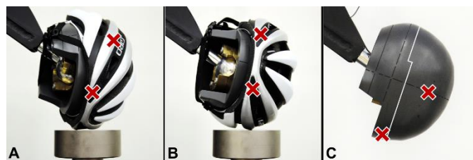
Figure 2.1 Headform orientation for (A) frontal and (B) temporal (above standard test lines) impact locations, and both locations on midsagittal view of ISO headform showing the impact test line in white (C). Locations were mirrored on the helmet and were a minimum of 120 mm apart, with the
