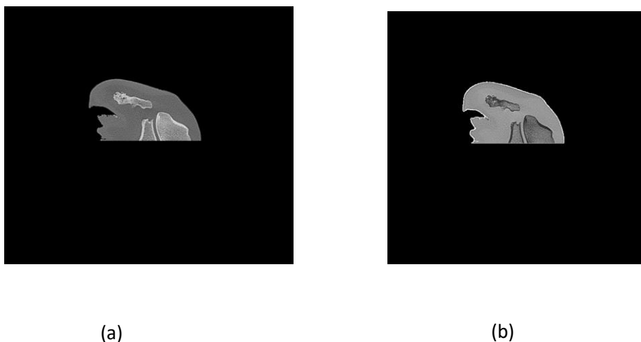
Figure 51: One of the Toolpath image set for fabrication of a continuous functionally graded part for fabricating cross-section model of horse leg a) Toolpath for material 1 b) Toolpath for material 2
