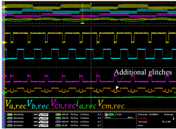
Fig. 4-20. Misalignments of switching instants by modification of carriers.
