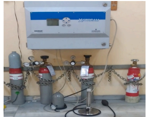
Fig. 4. Gas analyzer used for gas concentration measurements.
