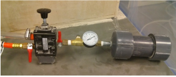
Fig. 2. Palm button charge and release valve system with air vessel.
