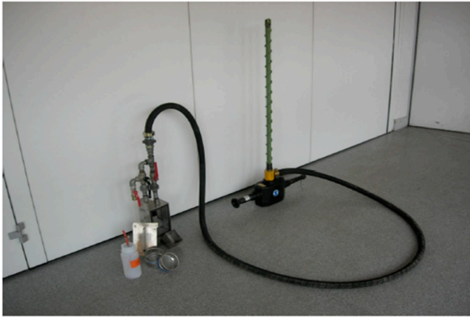
Fig. 2. Ejector and drilling machine for sampling
