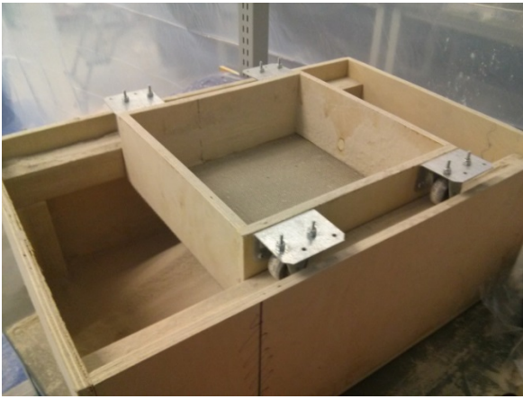
Fig. 6. Box screen-mesh assembly above dust layer.
