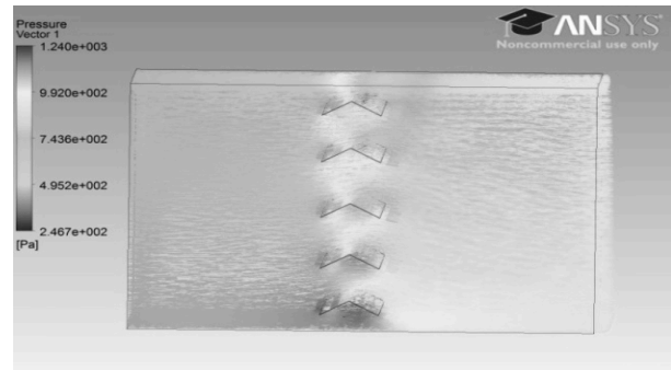
Figure 12. Pressure vectors across 0° angle louver.
