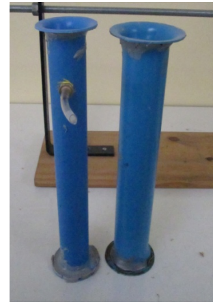
Fig. 3. Modified raise with curvature radius at PVC tube.
