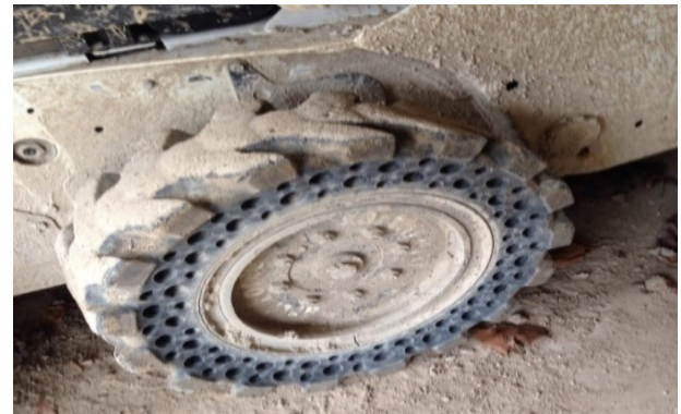
Figure 2. EarthForce™ solid press-on tire.
