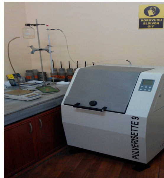
Fig. 5. Ring mill and burette assembly
