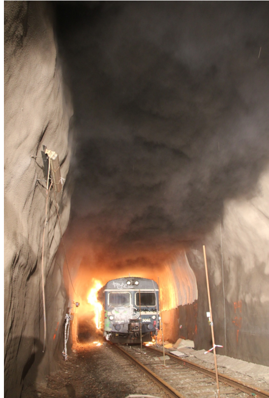
Fig. 1. Rollback occurring in a Swedish fire tunnel test [10].
