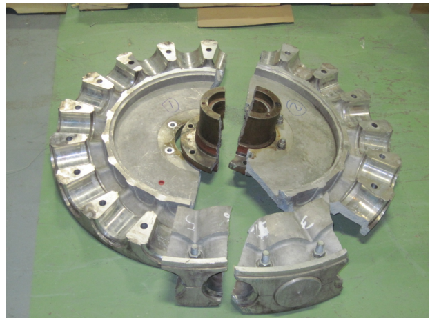
Fig. 2. Vertical fan no. 1 fractured fan hub and hub adapter.
