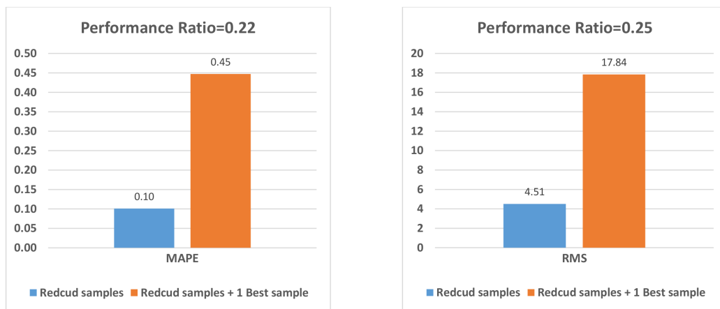
Figure 4.7. Performance of efficient-SBPF2 with and without forwarding the best sample in the resampling process.
