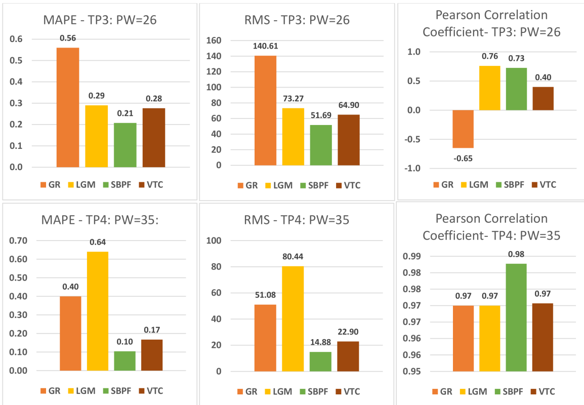
Figure 3.11. Error metrics: Pearson’s correlation coefficient, MAPE, and RMSE measure the direction and amount of deviation of short-term predictions of GRM, LGM, SBPF and VTC. Figures a, b, and c are the statistics corresponding to the third time point. Figures d, e, and f are associated with the fourth time point.
