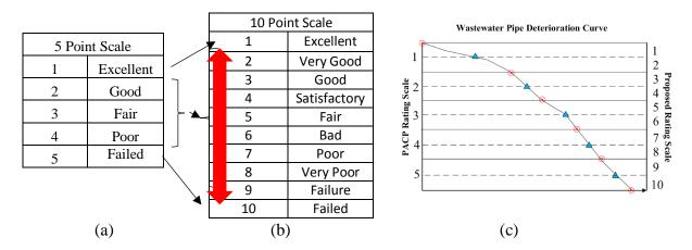
Figure 5-5. 5-Point Scale vs. Proposed 10-Point Scale for Performance Prediction
