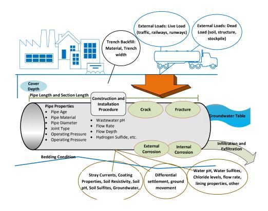
**Figure 1-1. Factors Effecting Wastewater Pipeline Performance**
