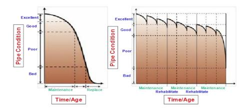
Figure 2-3. Condition/Performance Deterioration Prediction Model.
