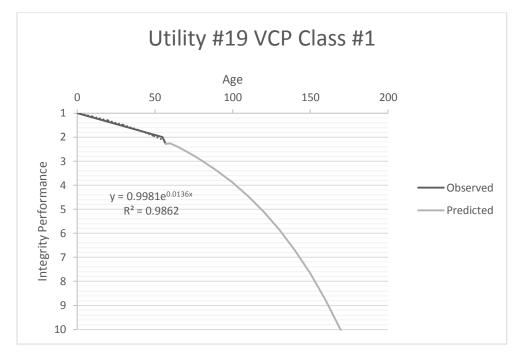
Figure G19-5. Time Dependent Model for Utility #19 VC pipe class #1 (collection, less than
