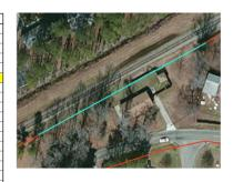
Index Output = 9 (Failing) Module = External Corrosion Reason = Presence of Railroad and Possible stray current
