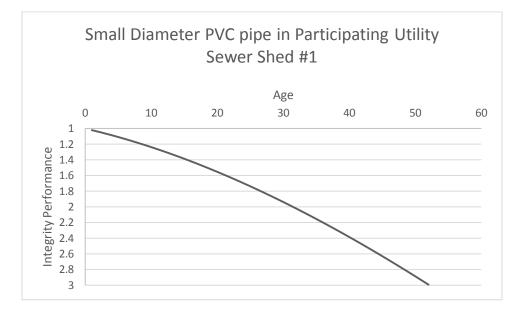
Figure G19-2. State Dependent Deterioration Model for Participating Utility
