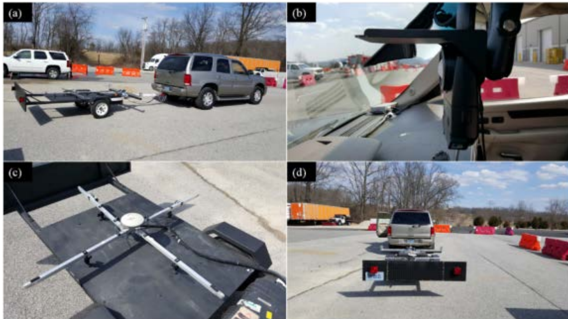
Figure 3. Photo. (a) TRLMMS hitched to vehicle. (b) Illuminance meter that measures the vertical illuminance mounted to the windshield. (c) “Spider” apparatus with GPS unit in the center. (d) TRLMMS from behind with the headlamp barrier that eliminates the influence of the following vehicle’s headlamps.
