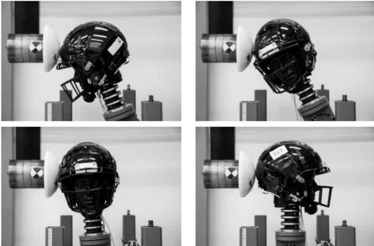
Figure 2.3: The front, front boss, side, and back locations tested on the pendulum impactor.
