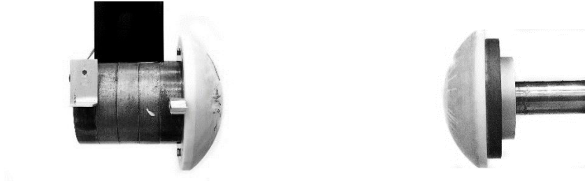
Figure 1.1: The pendulum impactor face (left) with a 20.3 cm rounded nylon impactor face, with a 12.7 cm radius of curvature; and the modified pneumatic ram impactor face (right) with a 1.24 kg nylon face, 5.5 kg steel disk, and 13.2 kg rod, with the same geometries as the pendulum impactor face. The effective impacting mass of both systems was 20 kg.
