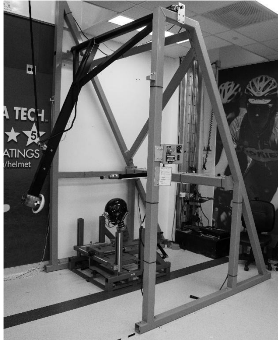
Figure 2.2: The pendulum impactor used for testing. The impactor was a 20.3 cm rounded nylon impactor face, with a 12.7 cm radius of curvature, mimicking the curve of a football helmet.
