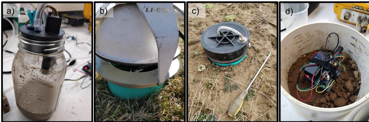
Fig 5.2: Measurement setups for: a) SMAAC-Biomass substrate induced respiration measurement; b) SMAAC-Field flux measurement with SMAAC simultaneously located within the LI-COR 8100 sampling chamber; c) SMAAC-Field flux measurement with SMAAC independent of the LI-COR unit; d) SMAAC-Burst laboratory CO 2 burst measurement.
