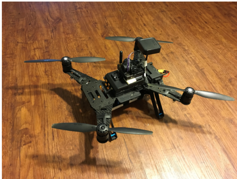
Figure 2.7: The Intel Aero drone, with optional indoor position sensor mounted on top
