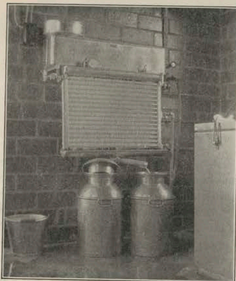
Double tubular cooler. Note that well water is used in upper half of cooler and refrigerated water in lower half. This method is economical and efficient
